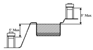
**NOTE:** If heater is installed outside of the limits shown, a flow switch must be used in place of the pressure switch when mounted and wired adjacent to the heater.
